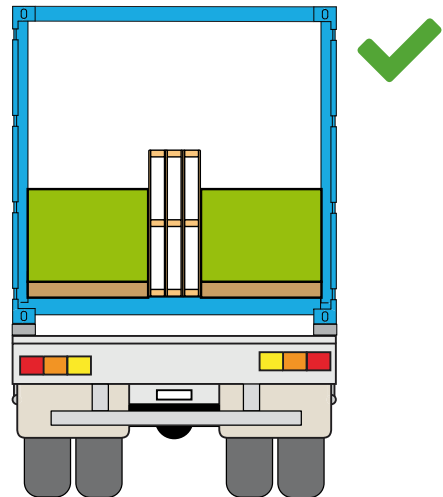
Gap filled with pallets
