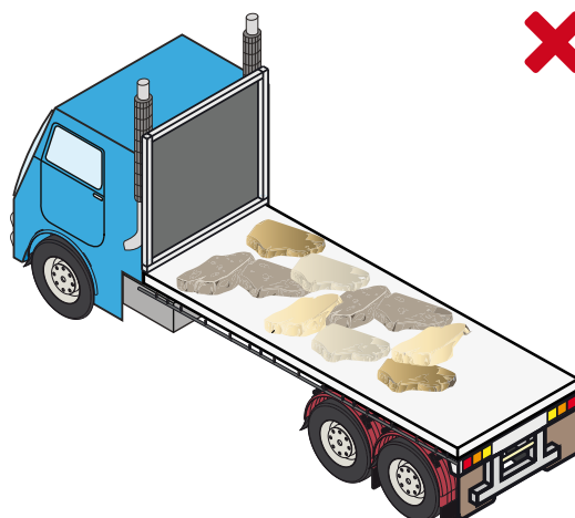
Figure 208 Loose bulk load – no containment
